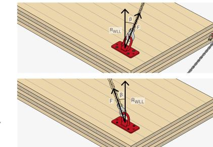
NOTE:  $\beta$  = lifting angle (angle between vertical axis and chain).
