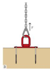
Connect the crane hook and carefully lift the timber element. Be careful about the allowed lifting directions and corresponding maximum lifting capacities.
