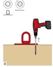
When lifting is complete, remove the screws and dispose of them. The screws can be used for only one handling cycle.
