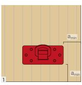
Read the instructions for use carefully and follow the directions. The positioning of the plate on the timber element must comply with the minimum distances.
